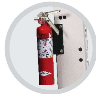
• Overhead Guard-Mounted Fire Extinguisher
