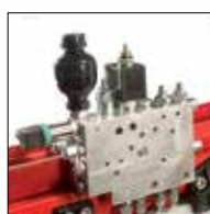
② Proportional valve Commands the hydraulic pressure in the clamping cylinders.
